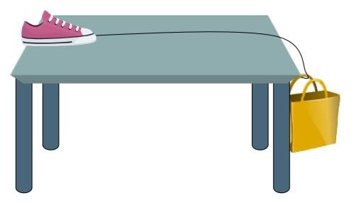
Make sure each shoe weighs the same by adding weights inside. Place a shoe at one end of the table. Attach the rope or string to the shoe. Attach the forcemeter or bag (hanging over the edge of the other end of the table) to the other end of the rope or string. Pull the forcemeter or add weights until the shoe keeps moving across the table. Record the measurement.
